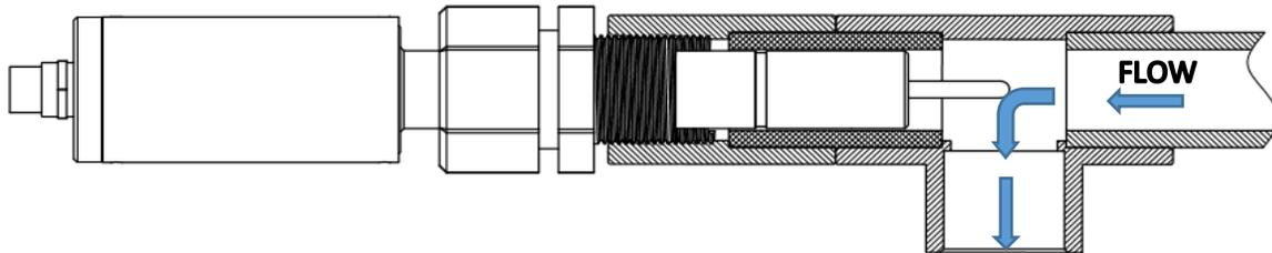
Figure 1. ECORR installation to the sample flow
