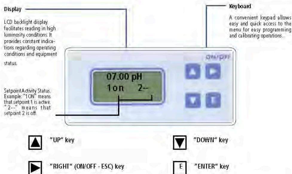
Into normal operating mode press "UP" or "DOWN" key for instrument's details.
